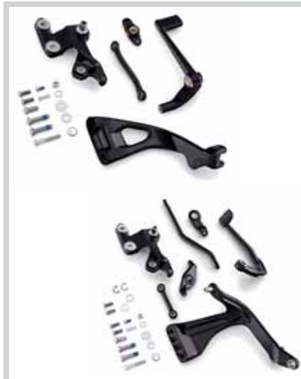
A. ORIGINAL EQUIPMENT MID-CONTROLS – BRAKE AND SHIFT SIDE
