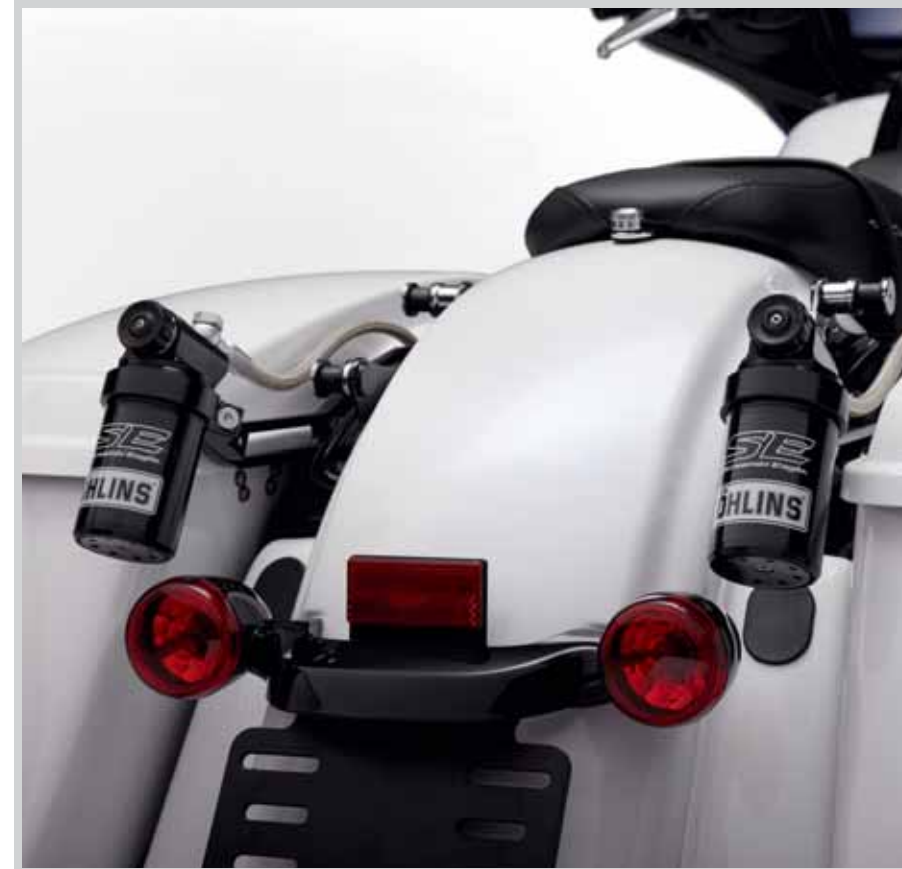
A. SCREAMIN' EAGLE®/ÖHLINS® REMOTE RESERVOIR REAR SHOCKS
