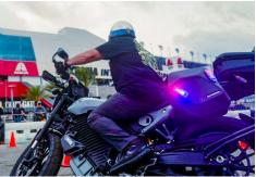
Upfitted with patrol-ready features, including lights, siren, top case, side carriers, hand controls, windshield and hand guards, the S2 Del Mar Patrol is built for duty. Riders can choose from four preset ride modes—sport, road, range and rain—plus two customizable modes defined by the rider. An adjustable suspension further enhances comfort and control, allowing for a tailored riding experience.
