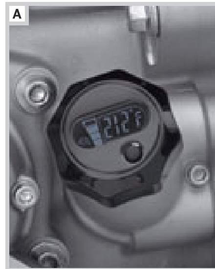
A. OIL LEVEL AND TEMPERATURE DIPSTICK WITH LIGHTED LCD READOUT – BLACK
