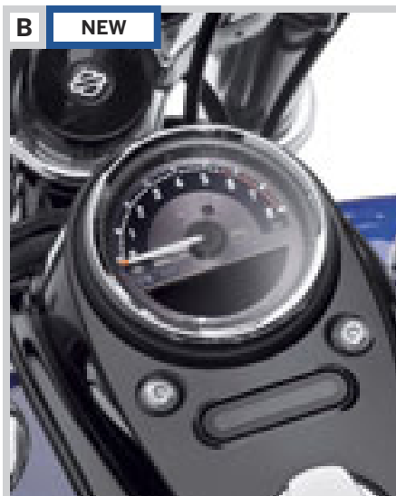
B. COMBINATION DIGITAL SPEEDOMETER/ANALOG TACHOMETER – 4" SPUN ALUMINUM DIAL
