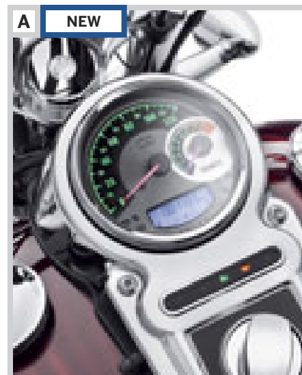
A. COMBINATION ANALOG SPEEDOMETER/TACHOMETER – 5" SPUN ALUMINUM DIAL
