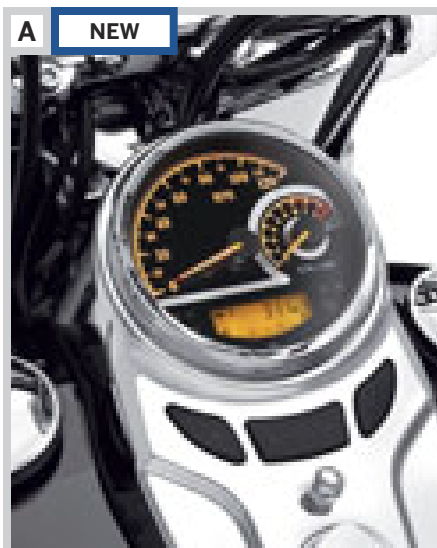
A. COMBINATION ANALOG SPEEDOMETER/TACHOMETER – 5" BLACK DIAL
